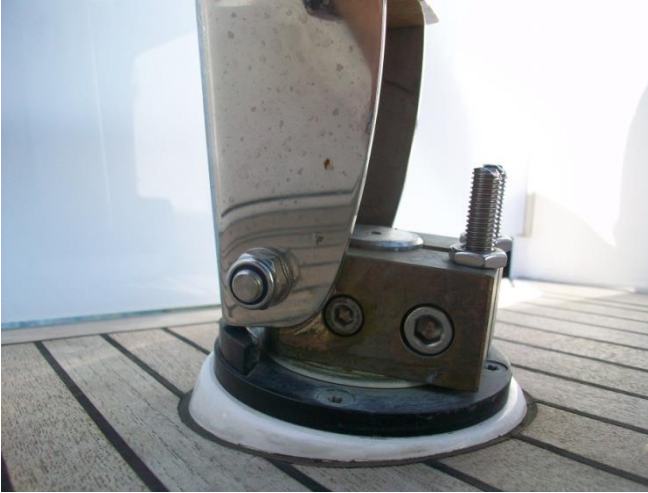
Hallberg-Rassy 310 upper rudder shaft fitting
