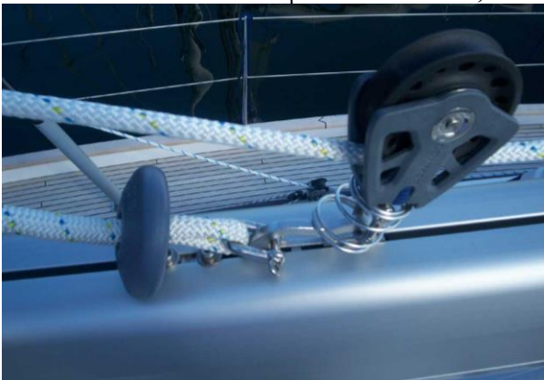
Incorrect position – will scratch the boom
