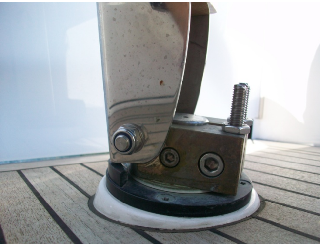
Hallberg-Rassy 310 upper rudder shaft fitting
